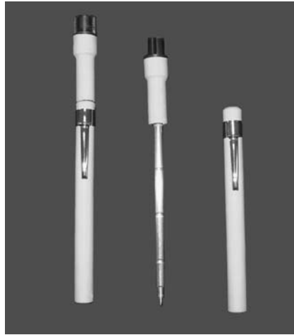
Figure 4. Pencil probe developed by the USDA/ARS/SWCRU for rapid field and laboratory analysis of electrical conductivity.
